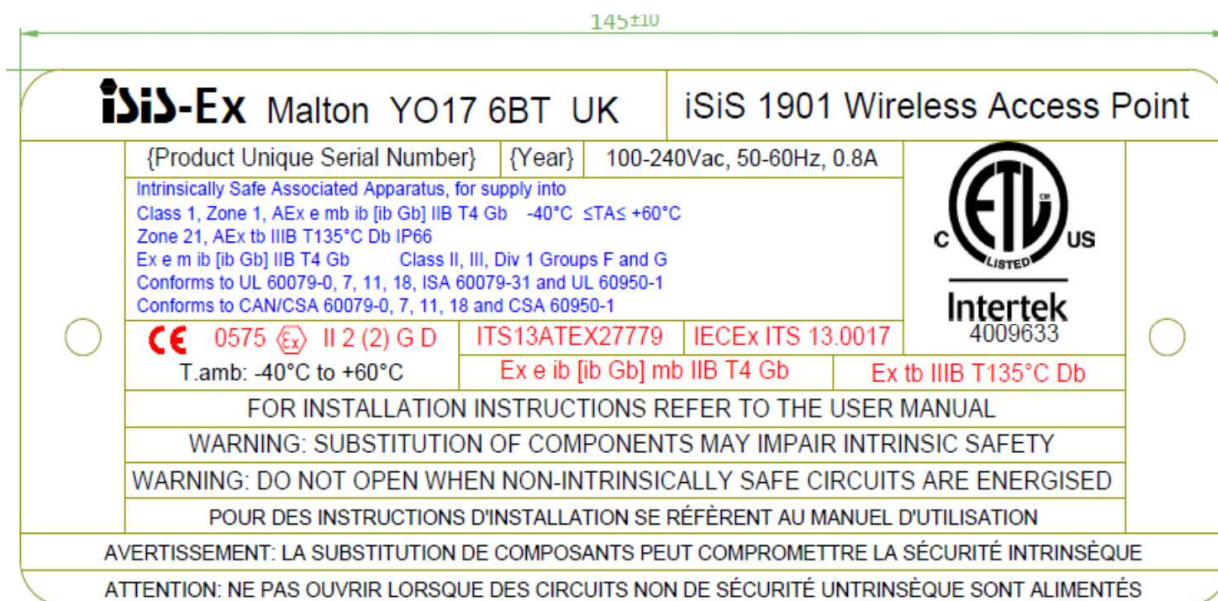
Illustration 2 - Ex Marking Label and Warning Marking
