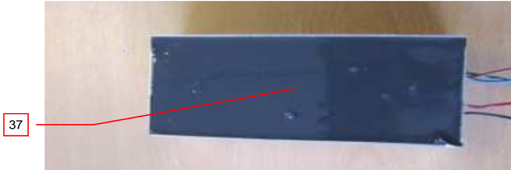
Photo 10 - Potted Power Supply unit, item 20
